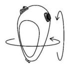
Rotate tank to ensure that all surfaces are kept wet with RustBlast. Repeat rolling and tipping tank every 5 minutes for a minimum of 20 minutes and until the tank surface is essentially rust free. DO NOT ALLOW RUSTBLAST TO DRY IN THE TANK.
