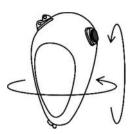
Let tank soak but always rotate it at intervals to ensure AquaKlean covers all surfaces. Heavy gum and varnish buildup may require extended soaking times up to 24 hours or more and/or the use of a pressure washer or agitation with media.
